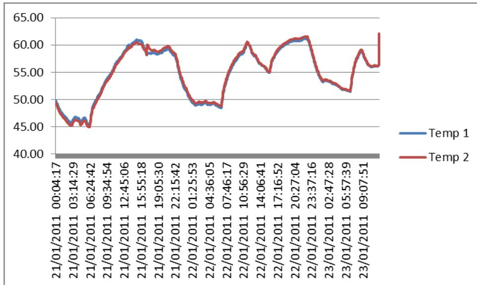
Temp. 1 refers to the temperature recorded on the first unit which has now been re-engineered using the CCWW restoration process incorporating pressure equalization, whilst the Temp. 2 refers to the temperature recorded on the standard (unchanged) unit. This clearly shows that the reengineering of the unit has a small but measurable improvement. The graph shows the effect of this over a period of 3 days.
