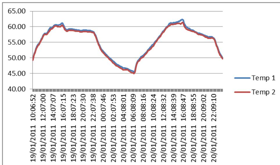
Temp. 1 refers to the temperature recorded on the first untreated unit, with the Temp. 2 referring to the temperature recorded on the second standard untreated unit. Graphs show virtually identical performance with variable temperature characteristics for the different times of the day.
