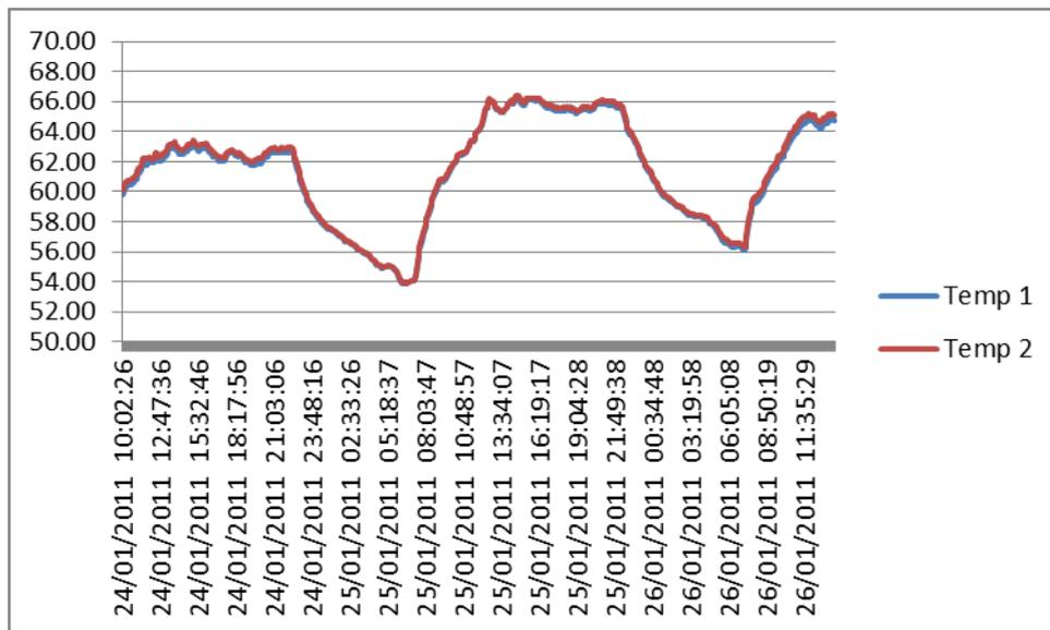
Temp. 1 refers to the temperature recorded on the Pressure Equalised Unit, whilst the Temp. 2 refers to the temperature recorded on the hitherto untreated unit which was now also equalized and resealed (removing the negative deflection but maintaining a permanent seal).
